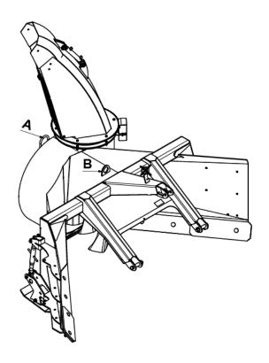
Transportation and management before use Snow blower housing is always lifted with strap attachments as illustrated. Please note that a single snow blower weigh is approx. 850 kg. Use lifting equipment suitable for this weight!!
